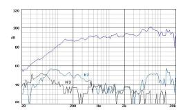
Note: on axis frequency response measured with loudspeaker standing on infinite baffle in anechoic chamber,  $1 \text{w} \otimes 1 \text{m}$ .
